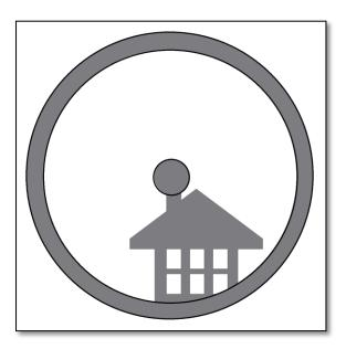
**4.3.** After playing with the twoadjusters and some trial and error we get the finderscope recticle close to the center (in this case the chimney). The finderscope is now ready to use!
